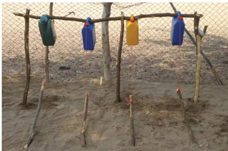
Tippy taps are set up for hand washing, as part of the UNICEF WASH in Schools programme in Benguela Province.
